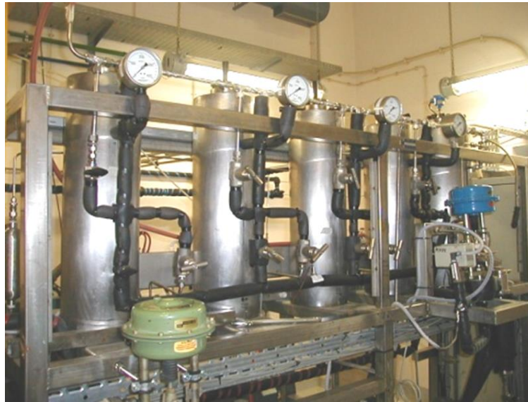
4 high pressure autoclaves of 1,8L each
